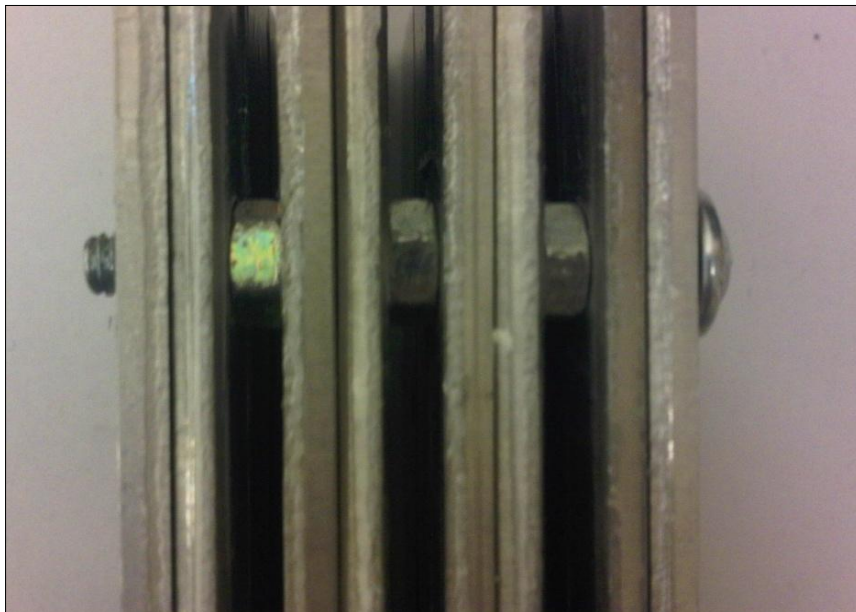
Figure 6.2 Top view of one of the aluminum stack configurations showing the through bolt and the spacing nuts.
